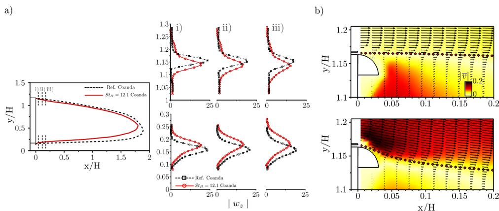
FIGURE 3 – a) Left : streamwise velocity iso-contour  $\bar{u} = 0.25$  for the unforced flow and for HF Coanda blowing ( $St_H = 12.1$ ). Right : evolution of the time-averaged vorticity along  $x$ . b) Upper shear layer zoom and transverse velocity field for the unforced flow (top) and HF Coanda blowing (bottom). Dotted points represent the streamlines originated from the exit slit.
