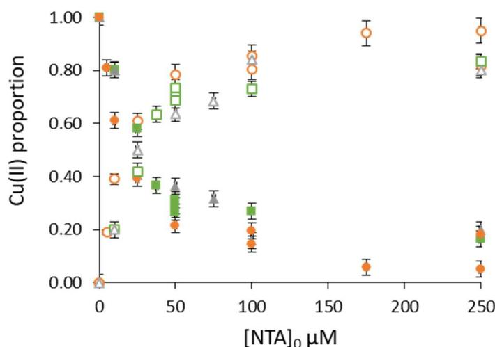
**Fig.5**  $Cu(II)$  proportion in  $A\beta_{1-16} - Cu(II)$  (plain symbols) or NTA -  $Cu(II)$  complexes (empty symbols) in 10mM Hepes, 15 mM NaCl, (●), 10 mM Hepes, 100 mM NaCl (■) 10 mM Hepes, 100 mM NaCl, 30 mM  $NaHCO_3$  (▲) as a function of NTA concentration
