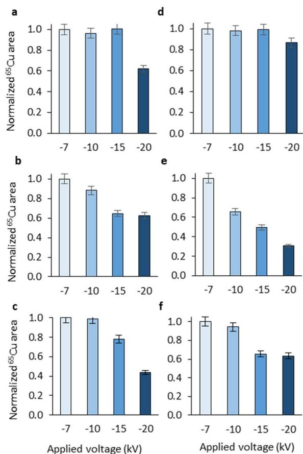
**Fig. 1** Voltage effect on AB - Cu(II) (a,b,c) and on NTA - Cu(II) (d,e,f) recoveries with Tris buffer and polybrene capillary (a,d) or Tris buffer and HPC capillary (b,e) or Hepes buffer and HPC capillary (c,f)
