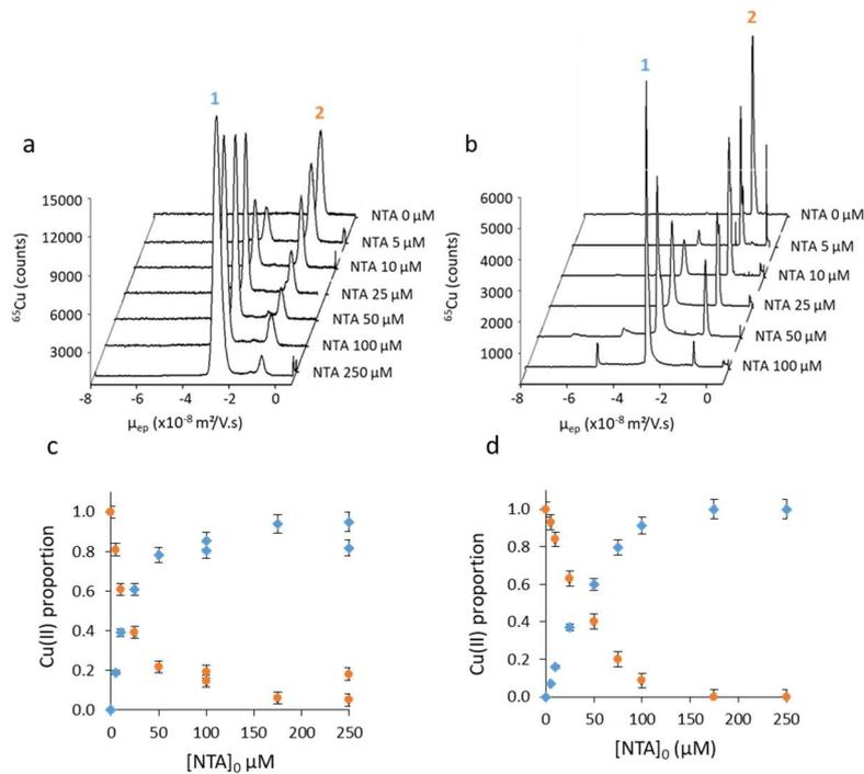
**Fig.4** Competition between  $A\beta_{1-16}$  and NTA for Cu(II) binding in Hepes buffer
