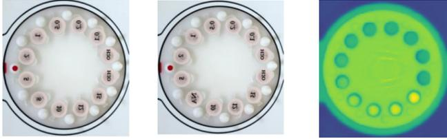
Fig.4. Two phantoms filled by different materials with different concentrations. Left: Phantom 1 filled by I. Middle: Phantom 2 filled by Gd (unit: mg/cc, NA indicates no filled material). Right: Original image of the 5<sup>th</sup> slice of Phantom 1 for the 1<sup>st</sup> energy bin.
