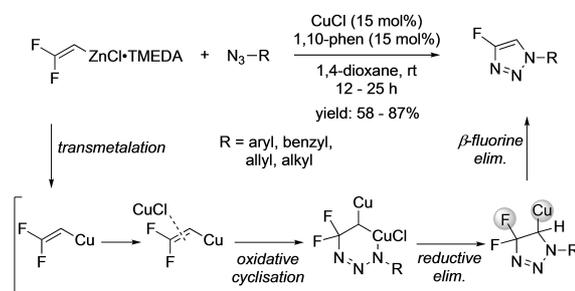
Scheme 9. Synthesis of 1-substituted 4-fluorotriazoles.
