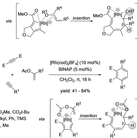
**Scheme 21.** Formal cross-alkyne cyclotrimerisation reaction using enol ethers and vinylic acetates as alkyne surrogates under rhodium catalysis.
