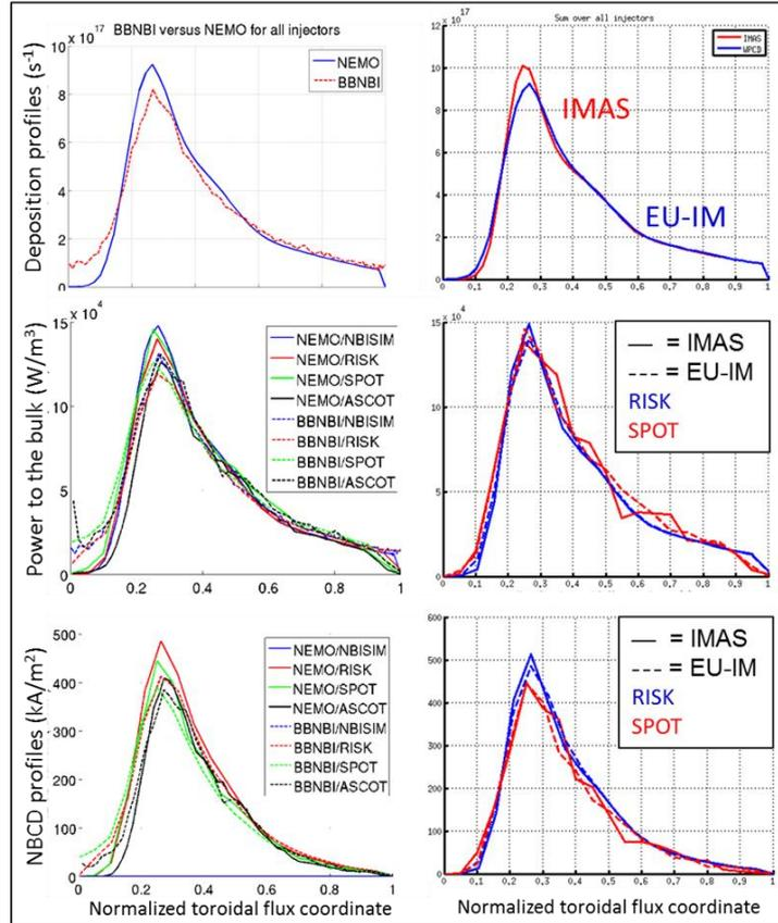
Figure 3: Result of the NBI benchmark using the H&CD workflow in EU-IM (left figures) and IMAS (right figures) frameworks for the ITER baseline scenario for the off-off neutral beam configuration. Top / middle / bottom figures show the deposition profiles, power to the bulk profiles and NBCD profiles respectively.
