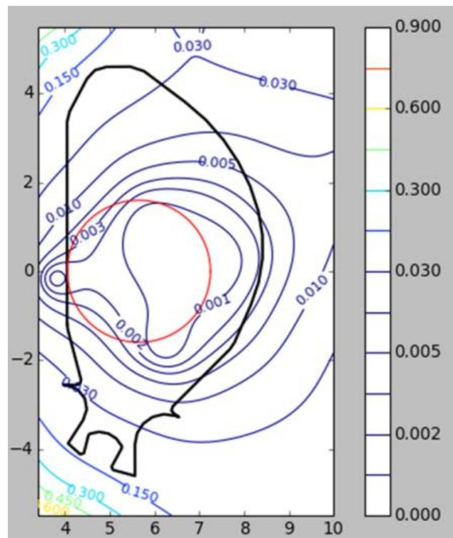
Figure 7: Magnetic field contours in ITER calculated for inboard start-up scenario
