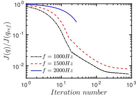
Figure 9: Convergence of  $J(q)$  towards a minimum value during the gradient descent optimization at three different input wave packet frequencies – and hence three different  $J(q_{ref})$ . In all cases,  $\lambda = 100$ . For  $f = 2000$  Hz, the optimization ended soon due to the  $|\tilde{\beta}(s)| \leq 1$  constraint being violated at 0 Hz. This is not the case for the other two frequencies, where computations are terminated manually after vanishing returns upon further iterations.
