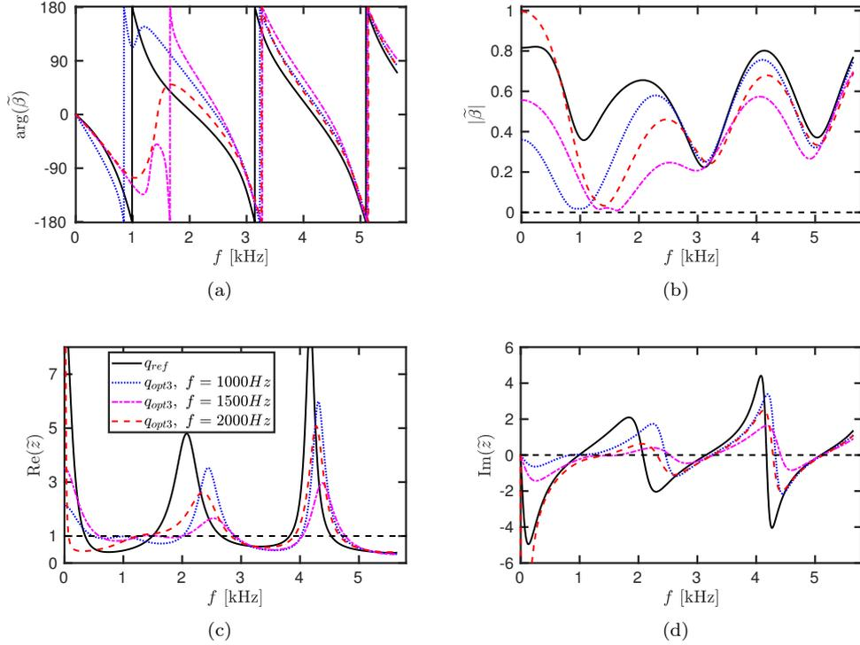
Figure 10: (a) Argument and (b) modulus of the reflection coefficient  $\tilde{\beta}(s)$  based on  $q_{ref}$  and  $q_{opt3}$  for the three analysed frequencies  $f$ . (c) Real and (d) imaginary part of the impedance  $\tilde{z}(s)$ .  $\tilde{z} = (1 + \tilde{\beta}) / (1 - \tilde{\beta})$ .
