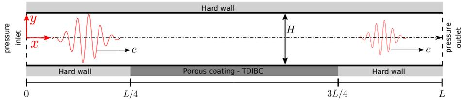
Figure 4: Sketch of the grazing incidence tube (GIT) test case.  $L = 812$  mm,  $H = 50$  mm. The right running pressure waves are damped under the effect of the TDIBC on the lower wall.
