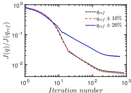
Figure 17: Convergence of  $J(q)$  towards a minimum value during the gradient descent optimization, with  $f = 1000\text{Hz}$  and  $\lambda = 100$  in all cases. Two convergence curves are obtained by perturbing each element of  $q_{ref}$  by a random factor of up to  $\pm 0.1$  (or  $\pm 0.2$ ) of its value.
