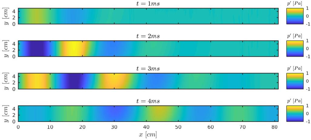
Figure 12: Plane wave packet evolution in the GIT test case, travelling at the speed of sound  $c = 344.37$  m/s towards the right. The TDIBC is located at the bottom wall, between  $20.3 \text{ cm} \leq x \leq 60.9 \text{ cm}$  – see Fig. 4. Simulation results obtained with the TDIBC parameters before optimization –  $q_{ref}$  shown in Table 1.
