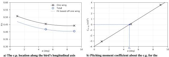
b) Pitching moment coefficient about the c.g. for the wing/body/tail combination, where  $\alpha_t$  indicates the trim angle
