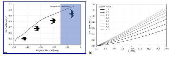
Fig. 10 Representations of a) lift coefficient in pullout illustrating different configurations, with M shape in the early pullout to open M at  $\Lambda_{\min}$  at the end of pullout; and b) effect of varying the aspect ratio A R on the theoretical lift coefficient.
