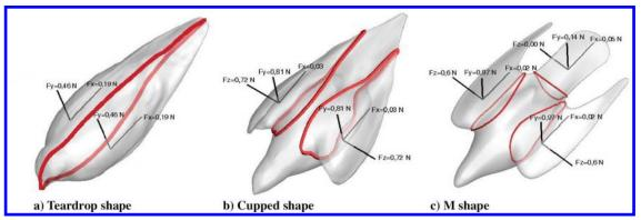
Fig. 4 Sectional aerodynamic forces over the falcon, the drag lift, and the side force represented as  $F_x$ ,  $F_y$ , and  $F_z$  respectively. All forces shown were taken at  $\alpha = 5$  deg.
