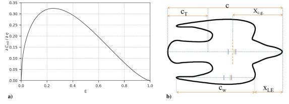
Fig. 8 Representations of a) change in pitching moment coefficient  $C_{M0}$  per angle of flap deflection  $\eta$  as given by Glauert [18]; and b) outline of model showing lengths and c.p. locations, at  $\alpha = 1,5$  and 9 deg respectively from left to right.
