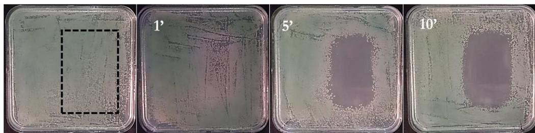
**Figure 11** Inactivation of large surface bacterial lawn composed of a mixture of three resistant strains with the multi spot plasma applicator applied in the zigzag scanning mode. H24 images of the inoculated sample exposed at H0 to 1, 5 and 10-minute plasma treatment. The dashed rectangle zone indicates the plasma treated region. The size of the treated zone is about 32 cm<sup>2</sup>.
