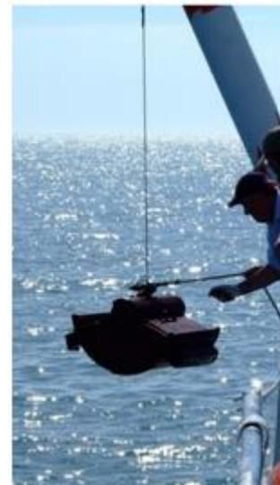
*Figure 10: Grab deployment from a RV.*
