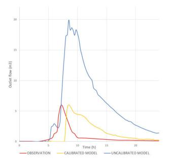
Figure 2. Comparison between calibrated and uncalibrated models in relation to observations on Floubalay
