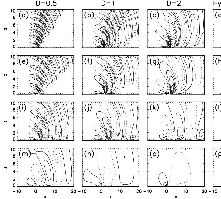
FIG. 1. Vertical velocity field for all simulation,  $S = 0.15$ . Each line corresponds to a value of  $J$ . The 3 columns on the left stand for different values of  $D$  and the column on the right is for the hydrostatic case with  $D = 1$ . In all panels, the contour interval  $CI = 0.004$  and the negative values are dashed.
