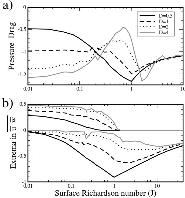
FIG. 4. Surface pressure drag (a) and minimum and maximum of Reynolds stress (b) for different slope  $S$  and  $D = 1$  in variable shear simulations. These two diagnostics are normalized by  $D_{rp}$  (Eq. (21)).
