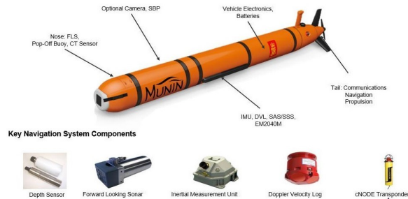
Fig. 2. The Kongsberg Mumin 1500 AUV and its components
