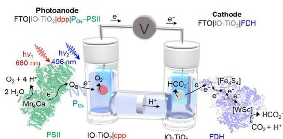
Figure 5 schematic view of the tandem cell used by Sokol and coworkers<sup>[82]</sup> to catalyze the photooxidation of water to O<sub>2</sub> at an anode incorporating photosystem II from *Thermosynechococcus elongatus* (left) coupled to the reduction of CO<sub>2</sub> to formate at a cathode
