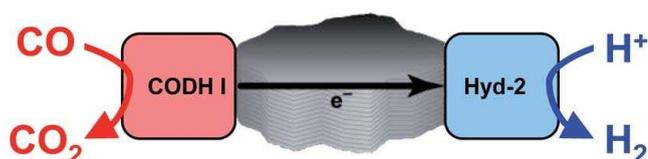
Figure 6: schematic representation of the graphite platelets used by Lazarus and coworkers to catalyze the water-gas shift reaction. CO is oxidized to  $\text{CO}_2$  by the CODH on the left, and the electrons generated are transferred via the graphite to the hydrogenase on the right, which produces  $\text{H}_2$ . Figure reproduced from <sup>[96]</sup> (Copyright © 2009 ACS, used with permission).
