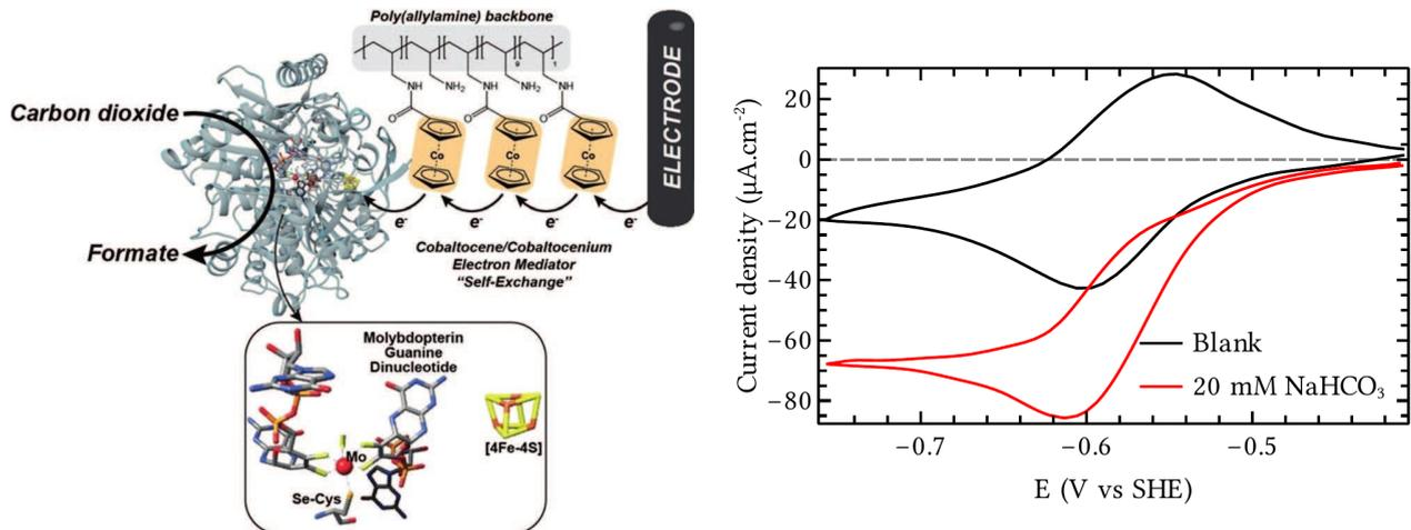
Figure 7: cobaltocene-based redox film incorporating *E. coli* FDH for the reduction of CO<sub>2</sub>. Left: scheme of the device, showing the electron transfer from the electrode to the FDH mediated by hopping across the immobilized cobaltocene moieties. Right: cyclic voltammograms showing the reduction of CO<sub>2</sub>. Data reproduced from <sup>[115]</sup> with permission.
