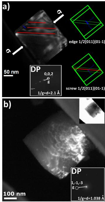
**Figure 2.** TEM images of nanocubes at different stages of *in situ* compression tests. (a) WBDF TEM image using the diffraction vector (002) of a 195 nm nanocube at yield stress. Crystallographic models are shown in the inset. (b) WBDF image of a 355 nm sized cube at zero load after 22% true strain (diffraction vector used  $\mathbf{g} = [1\bar{1}\bar{3}]$ ).
