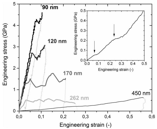
**Figure 3.** Experimental engineering stress-strain curves of MgO nanocubes of different sizes, all compressed along the [001] direction. The inset shows the onset of the curve for the 450 nm nanocube. Arrows indicate the lower and upper positions of the yield point used to determine the yield stress and its error bar.
