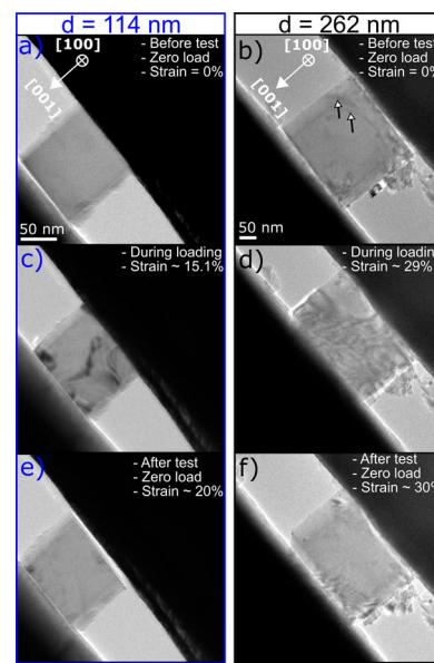
**Figure 1.** BF TEM images of  $\text{MgO}$  nanocubes (near [100] zone axis) extracted from compression tests along the [001] direction. (a,c,e) nanocube of size 114 nm before load, at  $\sim 15.1\%$  and  $\sim 20\%$  strain. (b,d,f) nanocube of size 262 nm before load, at  $\sim 29\%$  and  $\sim 30\%$  strain. Two dislocations are indicated by black arrows.
