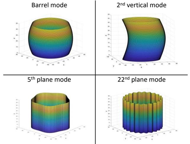
Figure 2. Illustration of some of the considered modes in the chosen basis description (amplitudes have been enhanced for more visibility)
