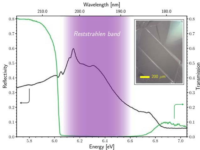
FIG. 2. Reflectivity (black) and transmission (green) of a high-quality hBN crystal, recorded close to normal incidence at 8 K. The crystal thickness is  $4.5 \mu\text{m}$ . The shaded area indicates the excitonic reststrahlen band in hBN. Inset: microscope image of high-quality hBN synthesized by the metal flux method.
