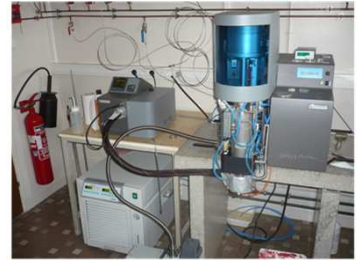
Photograph of the apparatus used for the thermogravimetry tests, without or with water vapor in air
