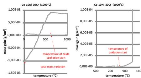
Example of plot of the mass gain versus temperature (here: T alloy oxidized at 1000°C in dry air)
