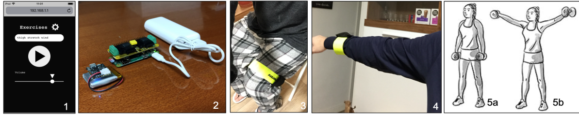
Figure 1. (1) User interface of the web application; (2) R-IoT with battery, and Raspberry Pi Zero with portable battery; (3-4) examples of a participant using the sonification band, when it was placed on their thigh (3) for squat, arm (4) for lateral raise (photos taken by the participants), and an example of calibration in which the start exercise position (5a) and end position (5b) are recorded and stored.
