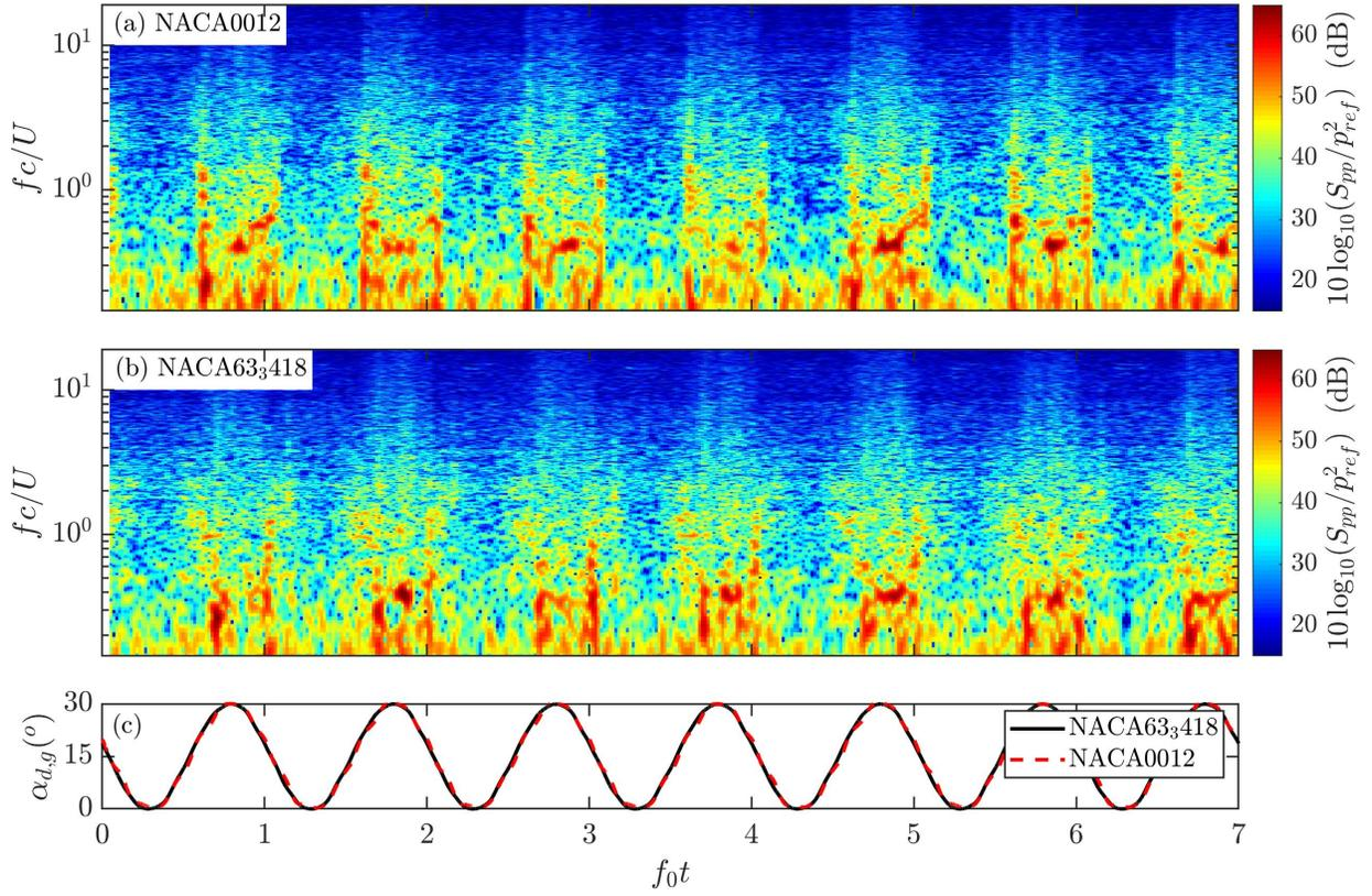
**Fig. 7** Instantaneous spectrograms of far-field acoustic pressure for (a) the NACA0012 and (b) the NACA63<sub>3</sub>418, and (c) instantaneous angle of attack for  $\alpha_{d,g} = 15^\circ + 15^\circ \sin(2\pi ft)$  and  $k = 0.01$ .
