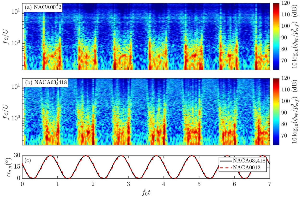
**Fig. 6** Instantaneous spectrograms of surface pressure at  $x/c = 0.92$  on the suction side for (a) the NACA0012 and (b) the NACA63<sub>3</sub>418, and (c) instantaneous angle of attack for  $\alpha_{d,g} = 15^\circ + 15^\circ \sin(2\pi ft)$  and  $k = 0.01$ .
