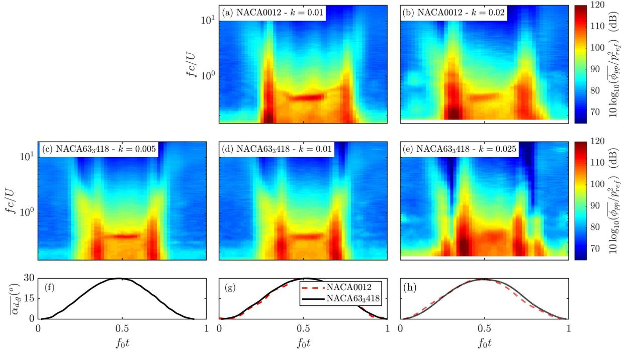
**Fig. 8** Phase-averaged spectrograms of surface pressure at  $x/c = 0.92$  on the suction side for  $\alpha_{d,g} = 15^\circ + 15^\circ \sin(2\pi f_0 t)$  for (a-b) the NACA0012 airfoil and (c-d-e) the NACA633418 airfoil, and (f-g-h) phase-averaged angle of attack. The overbar denotes phase-averaging.
