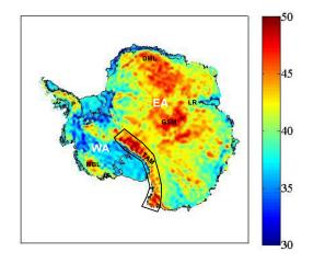
**Figure 5.** Estimation of crustal thickness (in km) from GOCE gravity observations. Geographical locations mentioned in the text are Dronning Maud Land (DML), Lambert Rift (LR), Gamburtsev Subglacial Mountains (GSMs), Transantarctic Mountains (TAMs), Marie Byrd Land (MBL) and the peninsula (P). The large TAMs separate East Antarctica (EA) from West Antarctica (WA).
