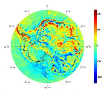
**Figure 1.** Free air anomalies in milligals (mGal) from the GOCE DIR5 solution.
