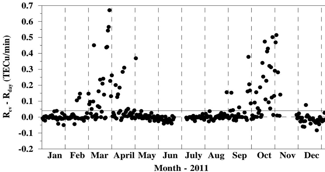
Figure 2. The variation  $R_{ev}-R_{day}$  at PHUT in 2011.  $R_{ev}-R_{day}$  values are presented by filled circles. The horizontal lines show 0.00 TECu/min and 0.04 TECu/min. The horizontal line at 0.04 TECu/min indicates the threshold for detection of ionospheric irregularity day
