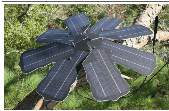
Figure 5: The RFCx Guardian acoustic sensor, equipped with eight solar panels and deployed in a tree. Photograph credit: Aya Naboulsi, Rainforest Connection.
