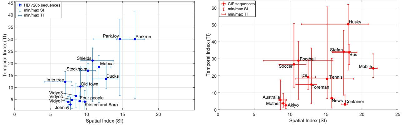
**Figure 3:** Illustration of the spatio-temporal index for the selected HD and CIF video sequences. Dots correspond to the average values across the video sequence. Vertical and Horizontal bars represent respectively the min/max value of the Temporal Index and the Spatial Index of the video sequences. From left to right: HD sequences, CIF sequences.
