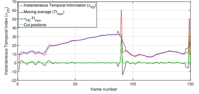
**Figure 9:** Example of the cut detection based on TI index for the *Tennis* sequence (cut on frames No.90, 149).
