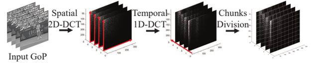
Figure 2: Compression Step in SoftCast scheme. From left to right: GoP in pixel domain, 2D-transformed frames, 3D-transformed frames, *chunks* division after 3D-DCT.
