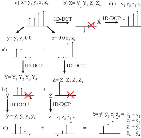
**Figure 8:** Illustration of the ghost effect phenomenon in the one-dimensional case considering 4 frames. a) and a') Vector of either pixels or 2D-DCT coefficients. b) and b') Resulting coefficients after temporal 1D-DCT; compression process in red. c) and c') Reconstructed coefficients after inverse 1D-DCT. The steps denoted by ' ) use the linearity property of the DCT.
