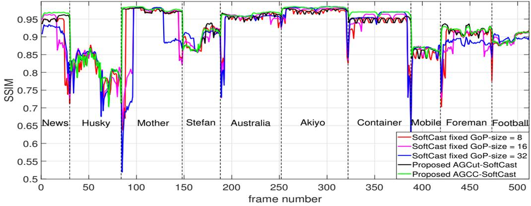
Figure 15: SSIM per frame for the *Mixed<sub>CIF</sub>* sequence, CSNR=15dB, CR=0.25 (75% of discarded coefficients).
