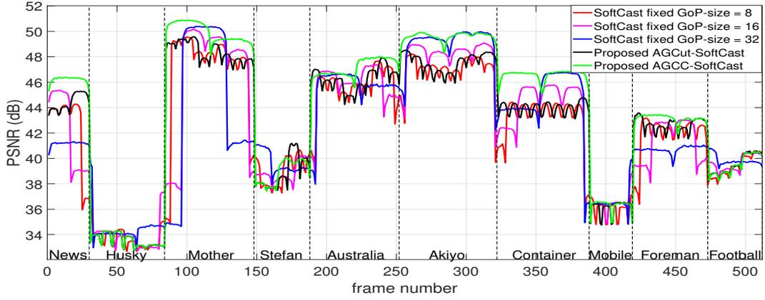
Figure 11: PSNR<sub>dB</sub> per frame for the *Mixed*<sub>CIF</sub> sequence, CSNR=15dB, CR=1 (no compression applied).
