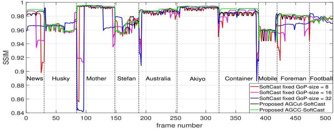
Figure 12: SSIM per frame for the *Mixed*<sub>CIF</sub> sequence, CSNR=15dB, CR=1 (no compression applied).
