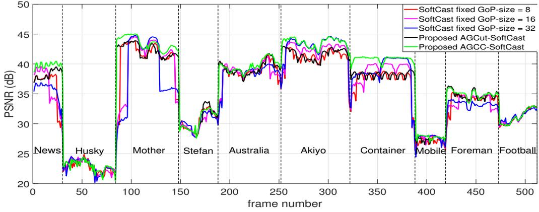
Figure 14: PSNR<sub>dB</sub> per frame for the *Mixed<sub>CIF</sub>* sequence, CSNR=15dB, CR=0.25 (75% of discarded coefficients).
