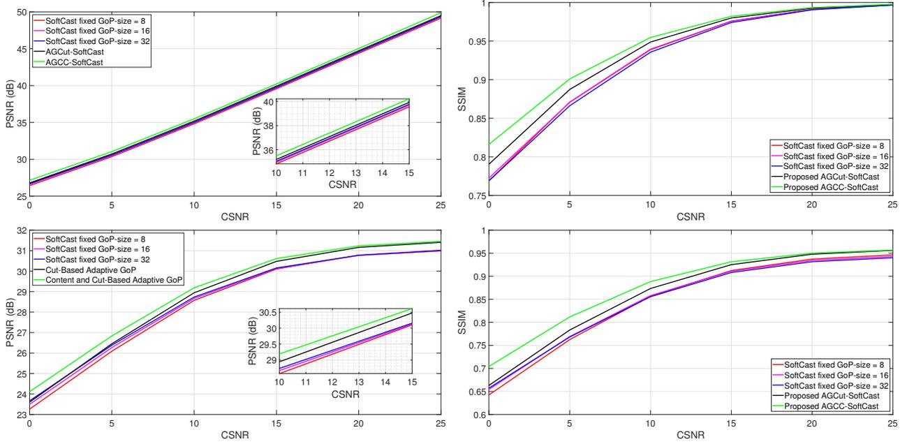
**Figure 16:** Average quality scores vs CSNR. First column: PSNR results. Second column: SSIM results. First row: CR=1. Second row: CR=0,25.
