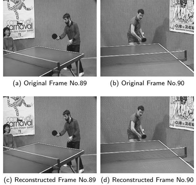
**Figure 7:** Ghost effect phenomenon, CR = 0.25, GoP-size=8. First row: Original frame No.89-90 of the *Tennis* sequence. Second row: Reconstructed frame after compression process (no transmission).
