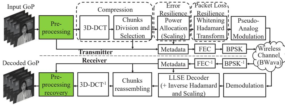
Figure 1: Block diagram of the SoftCast video transmission scheme.
