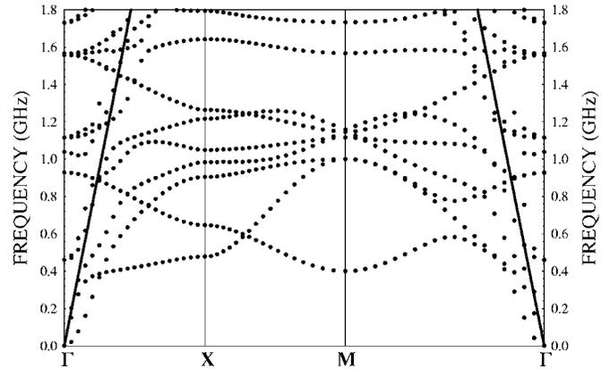
FIG. 5. Elastic band structures for the air/PZT phononic crystal plate of thickness  $h=a$  deposited onto a silicon substrate of thickness  $d=2h=2a$ . The thick solid lines represent the dispersion curves of the slower elastic waves propagating in an infinite, homogeneous medium composed of silicon, i.e., the waves of transverse polarization.
