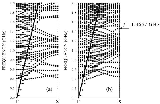
FIG. 7. Band structure along the  $\Gamma X$  direction calculated with a supercell containing  $1 \times 5$  unit cell, for (a) the perfect phononic crystal plate deposited on the silicon substrate and (b) the supported plate containing a waveguide formed by filling a hole in the third unit cell. The thickness of the substrate is the same as in Fig. 6, i.e.,  $d=5h=5a$ . The arrow indicates the location of the guided mode analyzed in Figs. 8(a) and 8(b).
