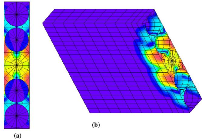
FIG. 8. (Color online) Maps of the modulus of the elastic displacement field for the waveguide mode with  $f=1.4657$  GHz at the X point in Fig. 7(b); (a) top view and (b) three-quarter view. The red color corresponds to the maximum displacement, whereas the blue color corresponds to the minimum.
