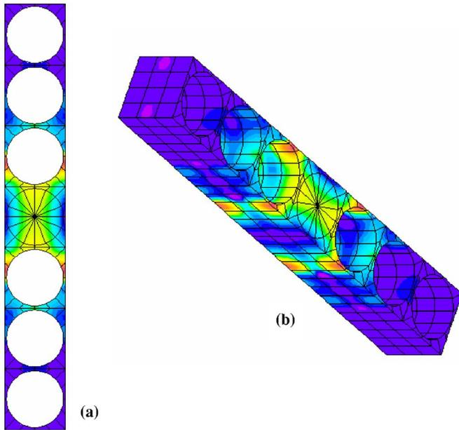
FIG. 4. (Color online) Maps of the modulus of the elastic displacement field for the waveguide mode with  $f=1.221$  GHz and a wave vector of modulus  $3.468 \mu\text{m}^{-1}$ ; (a) top view and (b) three-quarter view. The red color corresponds to the maximum displacement, whereas the blue color corresponds to the minimum.
