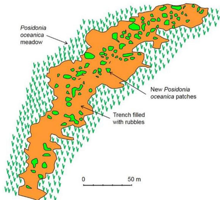
**Figure 8.** A trench dredged to set up a gas pipeline, then filled with rubbles in 2009, off the harbor at Ischia (Italy). Ten years later, 12% of the surface area of the trench had been spontaneously recolonized by *Posidonia oceanica*. From Cotugno et al. [161], redrawn and adapted.
