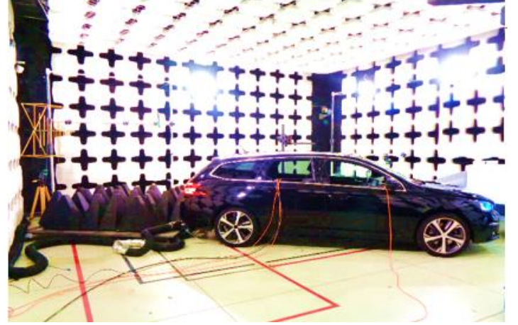
Fig. 6. Vehicle in the semi-anechoic chamber under radio test.
