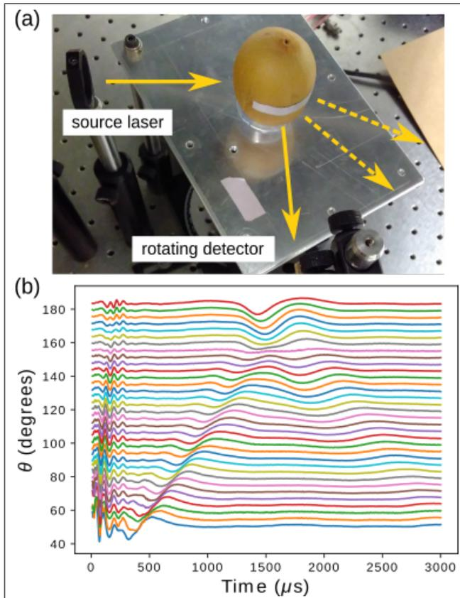
**Figure 2.** (a) Setup for LUS measurements on kiwifruit, in which the detector is rotated around the equator of the kiwi. (b) Example of data recorded with rotating detector setup. Plotted is the amplitude of transmitted waves as a function of angle between source and detector. In this plot, two waves can be seen: the P-wave at early times, and R-waves at later times.
