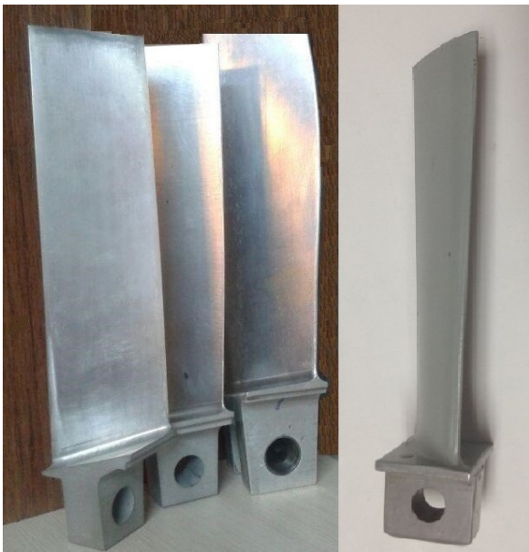
Fig. 5. The real machined turbine blades
