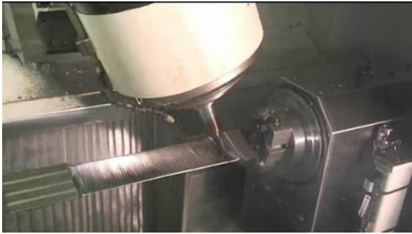
Fig. 4. Machining process of the turbine blades
