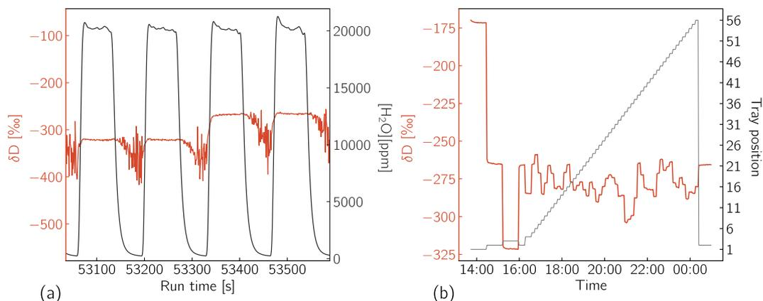
**Fig. 2** Vaporiser pulse example and run tray configuration. **(a)** A sequence of four vaporiser pulses focused at the transition from the “-40” to the “NEEM” standard water. **(b)** Vial tray configuration and raw  $\delta D$  data of a full measurement run as a function of time.
