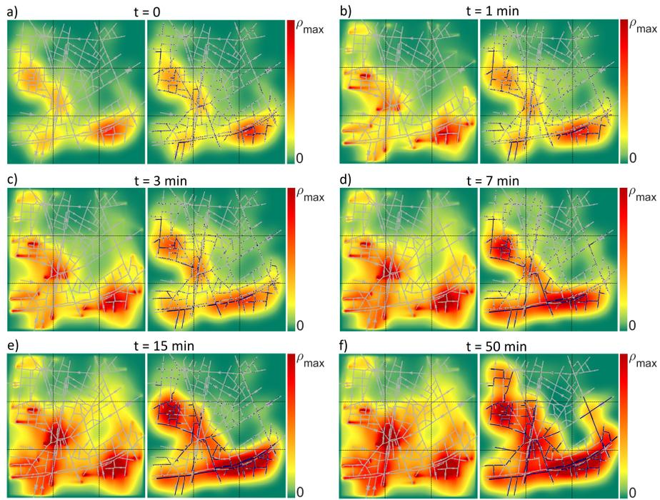
Figure 9: Congestion formation in Grenoble downtown for  $t \in [0, 50]$  min: numerical simulation of density governed by NEWS model (left plots) and Aimsun (right plots). Weighting parameter  $\eta = 20$ . Blue dots denote vehicle positions in Aimsun. Black dashed lines separate Grenoble in zones used for the calculation of SSIM.
