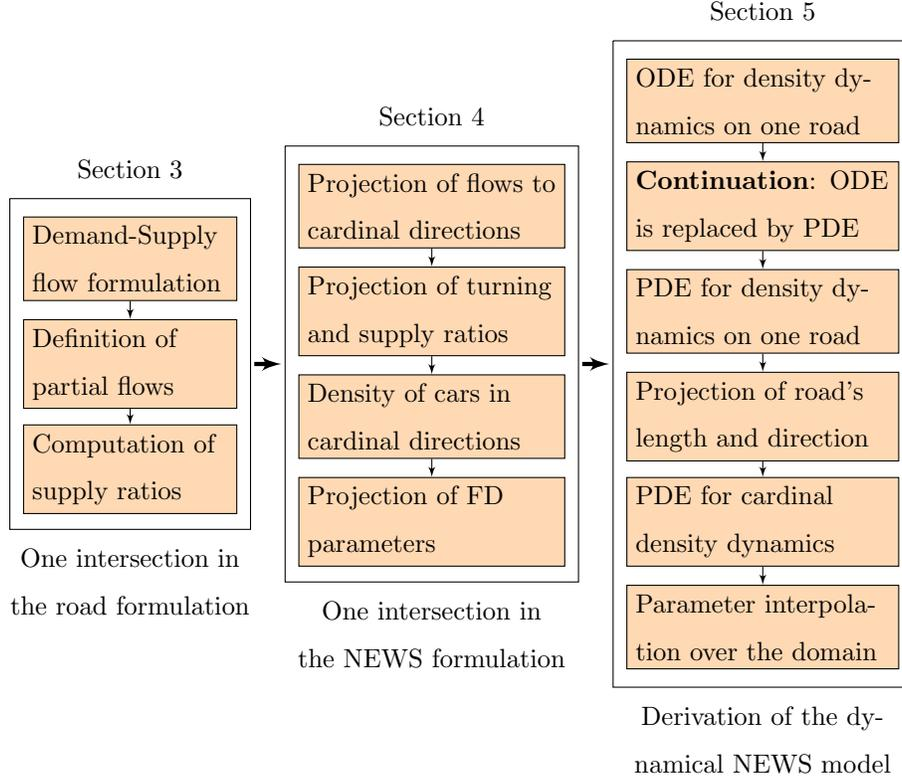
Figure 1: Workflow diagram of the derivation of the NEWS model.
