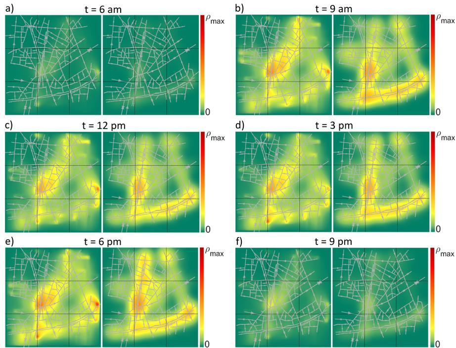
Figure 13: Evolution of traffic density in Grenoble downtown on 8th of January 2021 from  $t = 6$  am to  $t = 9$  pm: numerical simulation of NEWS model (left plots) and density estimated from sensor data (right plots). Weighting parameter  $\eta = 20$ .
