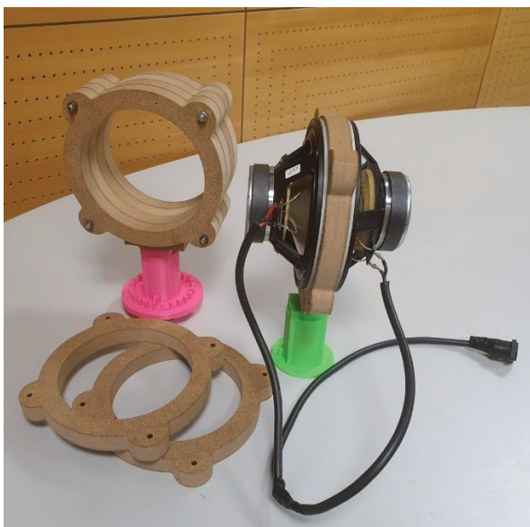
Figure 1. Prototype and parts explanation for coupled speakers omnidirectional sound source
