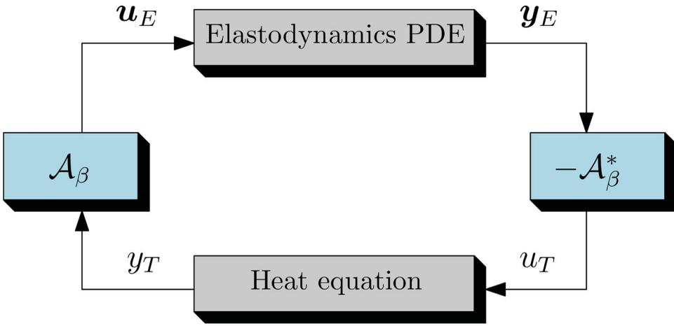
Figure 2. Schematic interconnection block diagram for linear thermoelasticity.
