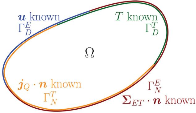
**Figure 1.** Boundary conditions for the thermoelastic problem, with 4 cases.
