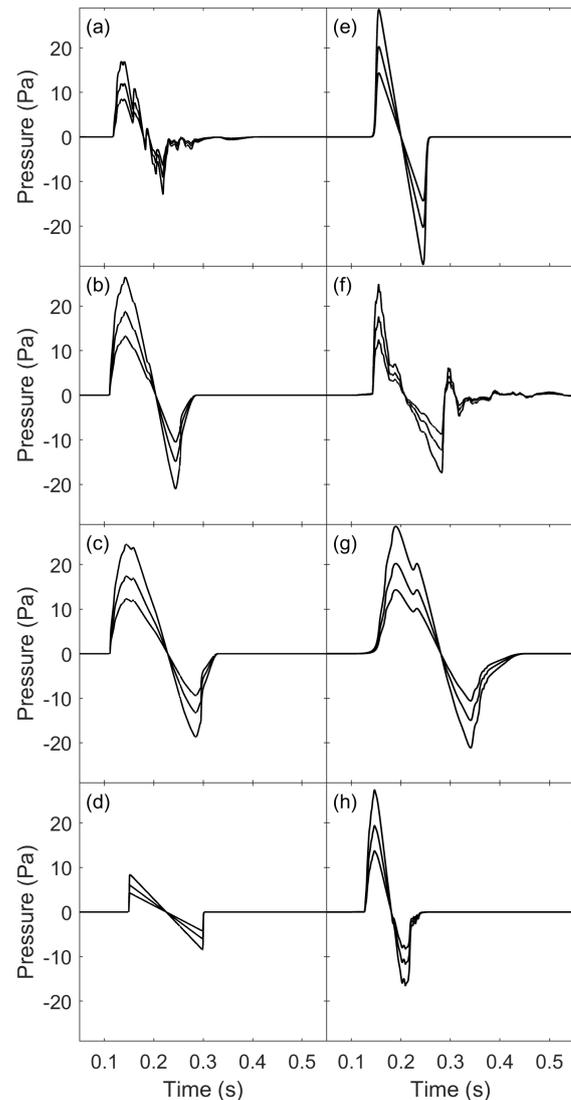
**Figure 2.** Time signals of the pressure for the eight different boom signatures used as input to the simulator. Each subfigure contains three curves for three different levels.
