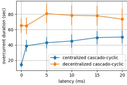
Fig. 10: Cumulative overcurrent duration versus telecommunication latency.
