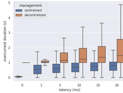
Fig. 11: Average overcurrent duration versus telecommunication latency.
