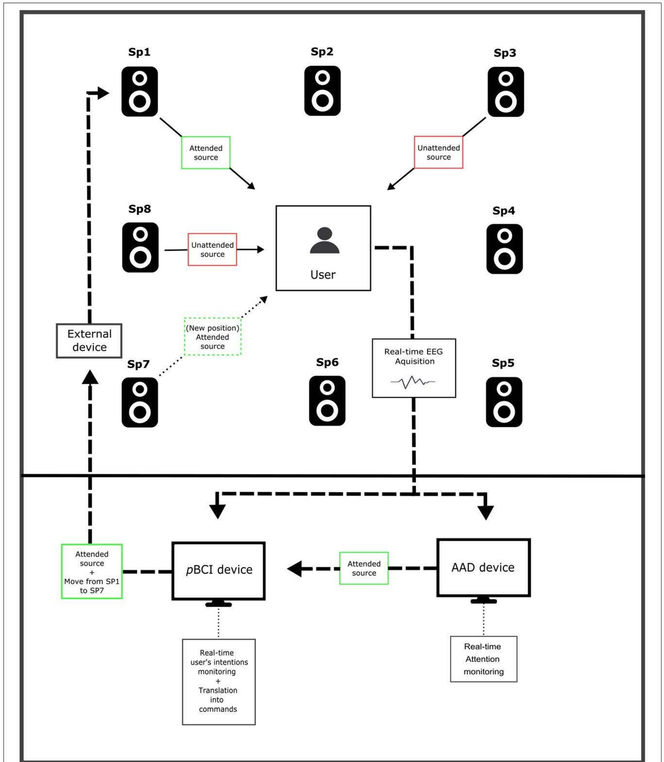
**FIGURE 2 |** Schematic representation of a real-time sound modulation AAD-pBCI system. Based on the real-time EEG data recording, the attended auditory source is continuously tracked by the AAD device. The pBCI device analyses in real-time the user's intentions (e.g., moving the attended source from the upper left loudspeaker to the bottom left one), translates it into commands and sends it to an external device that will modify the loudspeaker's parameters accordingly.
