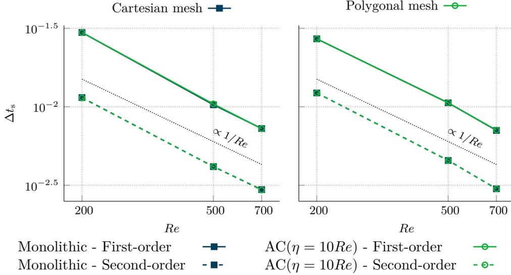
Figure 5: 2D Taylor–Green vortex. Critical time-step for stability,  $\Delta t_s$  (up to 1% resolution), as a function of the Reynolds number,  $Re$ , for several time-stepping schemes. Left: Cartesian mesh composed of 16,384 cells. Right: polygonal mesh composed of 15,129 cells.
