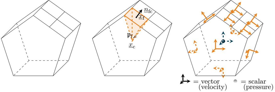
Figure 1: Mesh, notation and DoFs. Left: Example of a polyhedral cell with a hanging node. Center: The barycenter  $\underline{x}_c$  of the cell  $c$  and a face  $f \in F_c$  with its barycenter,  $\underline{x}_f$ , its normal  $\underline{n}_{fc}$  and its sub-pyramid  $\mathfrak{p}_{f,c}$ . Right: Full set of velocity and pressure DoFs for the considered cell (dashed arrows are used for velocity DoFs on hidden faces).
