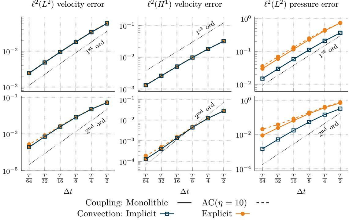
Figure 2: 2D Taylor–Green vortex. Convergence results for the space-time velocity and pressure errors.  $Re = 1$ ,  $T = 1.2$ . Top: first-order schemes; bottom: second-order schemes. Cartesian mesh composed of  $512^2$  cells.
