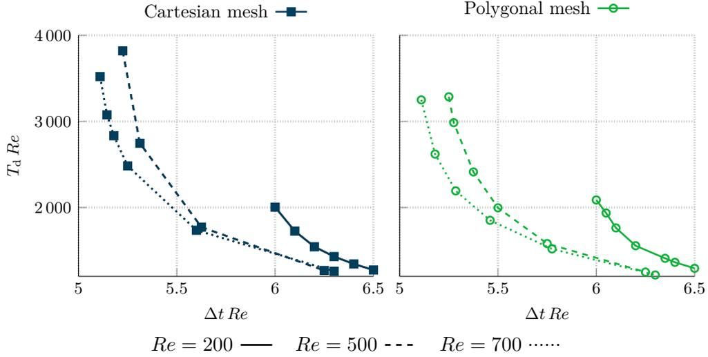
Figure 4: 2D Taylor–Green vortex. Monolithic approach and explicit convection. Divergence time  $T_d$  (scaled by  $Re$ ), for different choices of  $\Delta t$  (scaled by  $Re$ ). Left: Cartesian mesh composed of 16,384 cells. Right: polygonal mesh composed of 15,129 cells.
