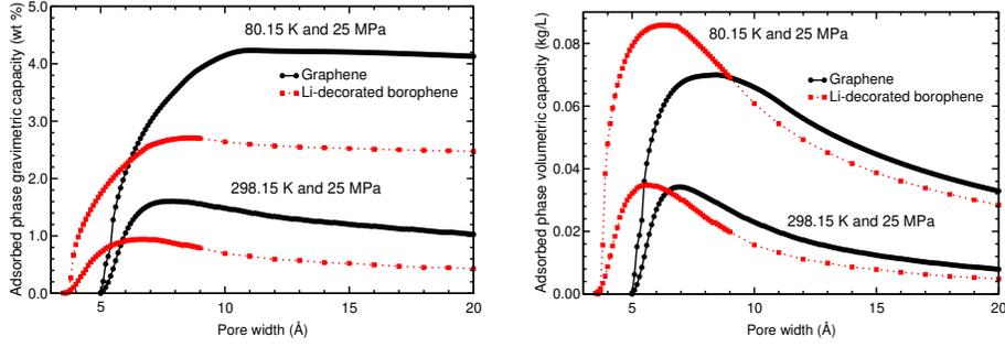
**Fig. 6.** Gravimetric and volumetric hydrogen storage capacities of slit pores of Li-decorated  $\beta$  borophene (red curves), as functions of the pore width, for 80.15 K and 298.15 K, and a pressure of 25 MPa. Capacities for graphene slit pores are also shown (black curves).
