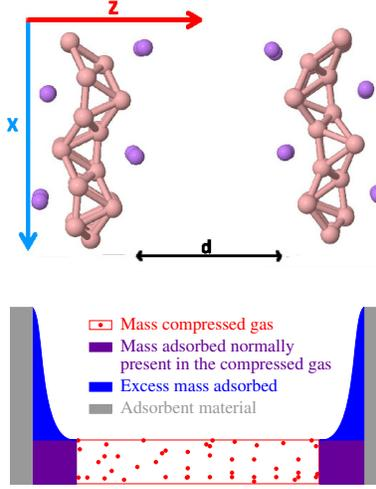
**Fig. 3.** Upper panel: Geometrical structure of a Li-decorated borophene slit pore of width  $d$ , made of two parallel Li-decorated  $\beta$  borophene sheets. Lower panel: Schematic representation of the phases of hydrogen stored inside a slit pore.
