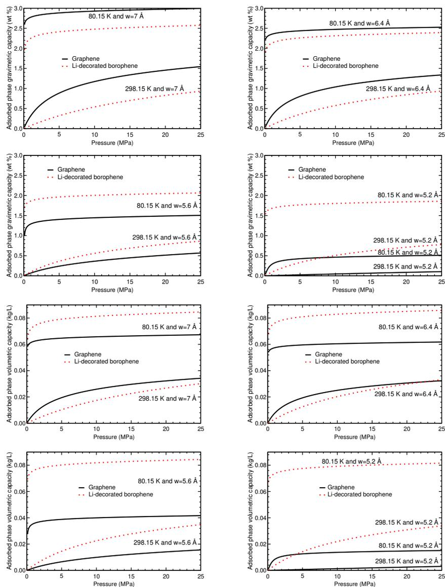
**Fig. 8.** Gravimetric (upper panels) and volumetric (lower panels) hydrogen storage capacities of the Li-decorated borophene slit pore (red curves), as a function of pressure, at 80.15 K and 298.15 K, for pore widths of 7, 6.4, 5.6 and 5.2 Å. Capacities of graphene slit pores are also shown (black curves).
