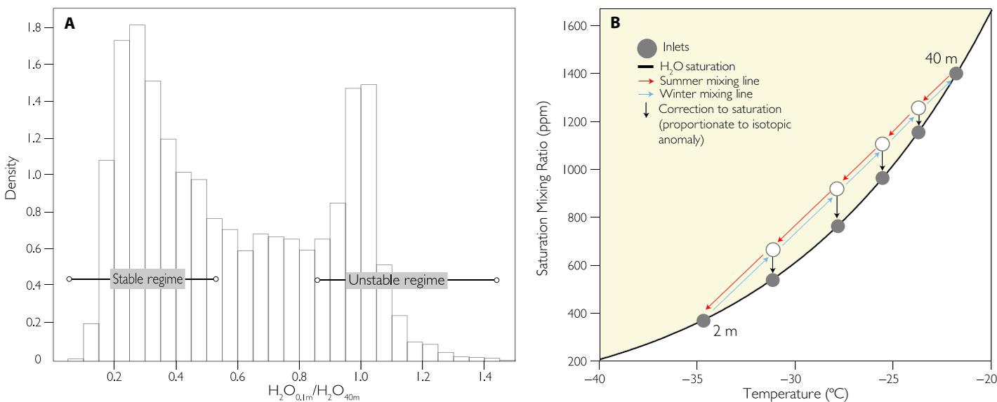
**Fig. 1. Humidity profiles over Summit Camp.** (A) Distribution of the ratio between the water vapor mixing ratio at the surface (~0.1 m) and at ~40 m taken from hourly averaged profiles between 2012 and 2014. (B) Saturation mixing ratios as a function of temperature (47). Theoretical summer and winter mixing lines with schematic depictions of where the air inlets in Fig. 2 would be sampling.
