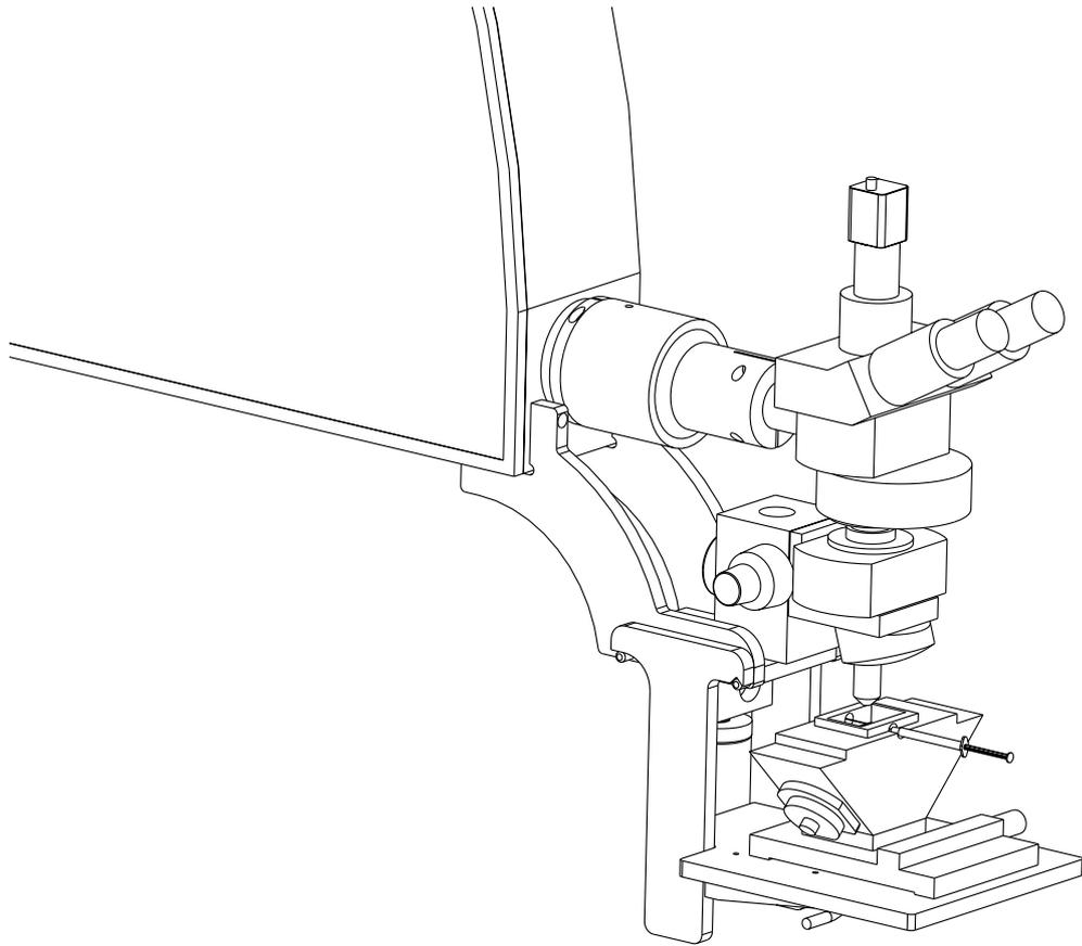
Figure 4: Line drawing of the optical observation part of the Brandaris-128 system.
