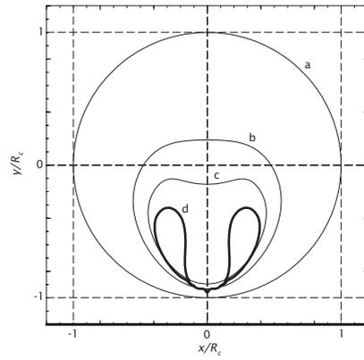
Figure 1: Schematic evolution of jet development in a collapsing bubble near a boundary (below): bubble on the verge of collapse (a), asymmetric collapse (b), jet development (c), funnel-shaped protrusion (d).
