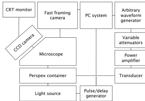
Figure 2: Basic setup of the high-speed photography system.
