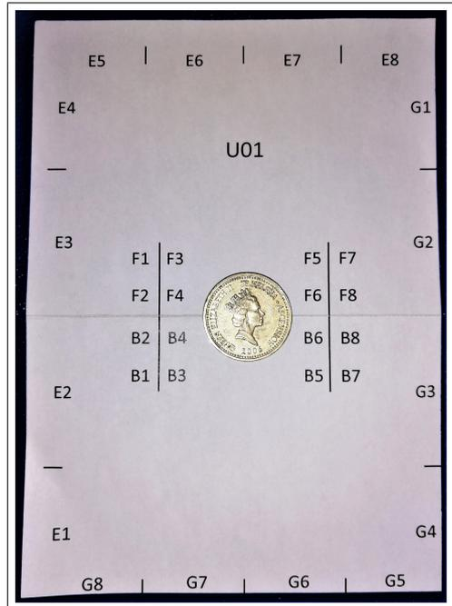
Figure 4: A6-sized experimental sheet with marks indicating the industrially cut edge (E1-E8) and along the incisions (F1-F8).
