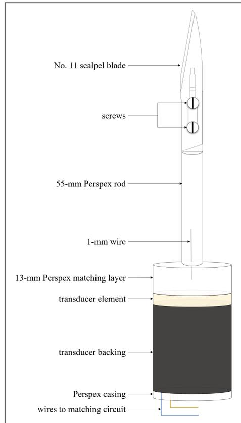
Figure 2: Ultrasonic cutting device with a single element ultrasound transducer and a scalpel blade attached with screws to a 55-mm Perspex rod.
