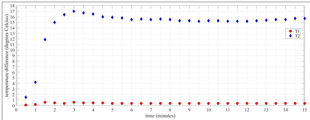
Figure 5: Temperature difference over a 15 minute period with the ultrasonic knife under sonication. The red dots indicate the temperature difference at the blade (T1) and blue diamonds indicate the temperature difference over the ultrasound transducer (T2).
