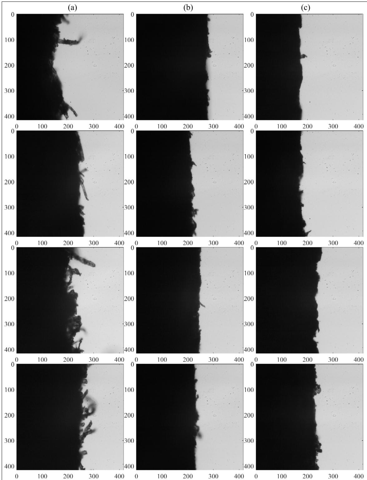
Figure 6: Back-lit bright-field 10 $\times$  microscopy images of incisions in paper from an unsonicated blunt blade (a) and a sonicated blunt blade (b), compared to the paper edge from sharp industrial cutting (c). The dark areas represent the paper. Each frame corresponds to a  $416 \times 416 (\mu\text{m}^2)$  area.
