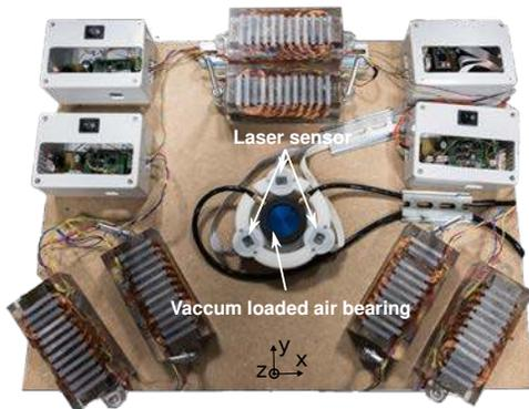
Fig. 5. Air bearing and position sensor system.
