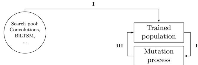
Fig. 1: **I.** Architectures are constructed with randomly sampled operations and then trained and evaluated, **II.** Sample randomly 10 architectures, and rank them by Precision@5. The most performing one is selected for mutation, **III.** The newly mutated architecture, is trained and evaluated. Then placed in the trained population. The oldest architecture is removed from the population.
