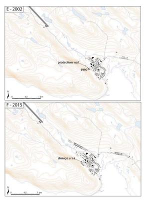
Dates and further runout of snow avalanches are marked with an asterisk, as well as the position of the 150 m long by 5 m high protection wall erected behind the former school and gymnasium, now used as a storage area. Buildings in grey on the F-2015 map are those build between 2015 and 2019.
