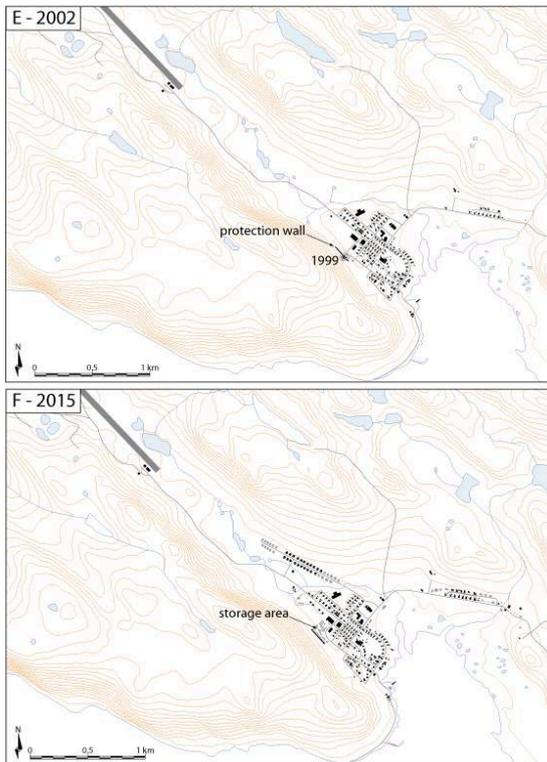
Dates and further runout of snow avalanches are marked with an asterisk, as well as the position of the 150 m long by 5 m high protection wall erected behind the former school and gymnasium, now used as a storage area. Buildings in grey on the F-2015 map are those build between 2015 and 2019.
