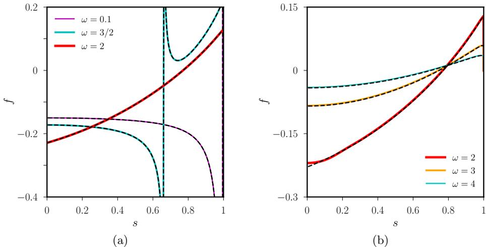
FIGURE 4. Rotation rate of the mean zonal flow, as a function of the cylindrical radius  $s$ , in rotating spheres subject to weak longitudinal librations (with  $\Omega_0 = 0$ ,  $m = 0$ ). (a) Our analytical results (solid coloured curves) are compared with the theoretical results (black dashed curves) of Sauret & Le Dizès (2013). (b). Comparison between the theory (black dashed curves) and DNS (solid coloured curves) at  $E = 10^{-7}$  and  $\epsilon = 10^{-4}$  when  $\omega \geq 2$ .
