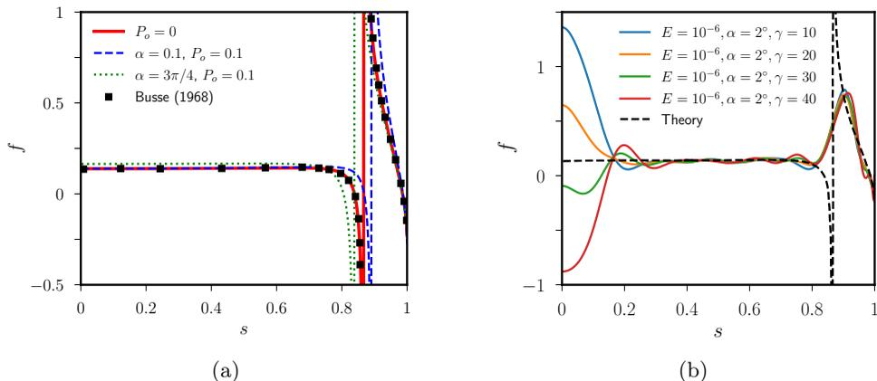
FIGURE 7. Rotation rate of the mean zonal flow, as a function of the cylindrical radius  $s$ , for a precessing sphere. (a) Comparison of theoretical profiles between our theory and Busse’s predictions (black squares, extracted from figure 1 in Busse 1968*b*). (b) Comparison between our theory (black dashed curve) and DNS (solid curves) for different values of  $P_o$  with  $\gamma = P_o/E^{1/2}$ .
