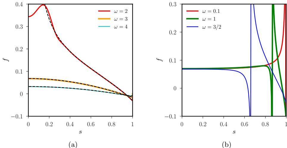
FIGURE 6. Rotation rate of the mean zonal flow, as a function of the cylindrical radius  $s$ , for a rotating sphere subject to weak latitudinal librations. (a) Comparison between theory (black dashed curves) and DNS (coloured solid curves) at  $E = 10^{-7}$  and  $\epsilon = 10^{-4}$  in the regime  $\omega \geq 2$ . (b) Theoretical zonal flows when  $\omega < 2$  with divergent flows at the critical latitudes.
