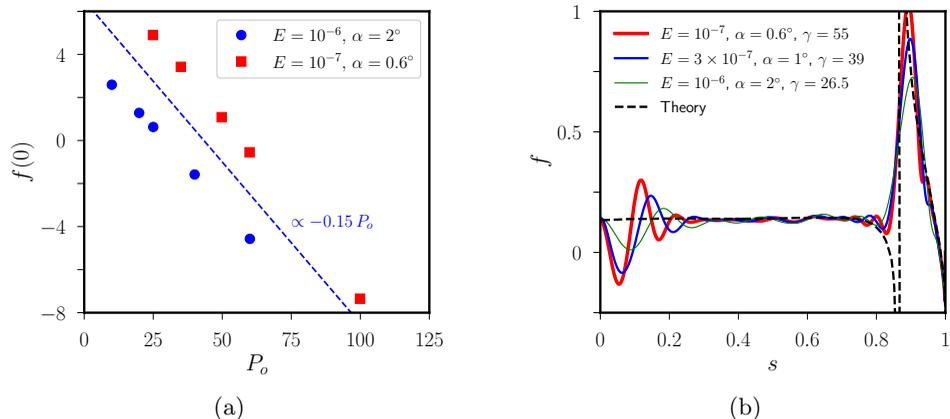
FIGURE 8. Mean zonal flows driven by precession in spheres. (a) Value at  $s = 0$  of  $f$ , as a function of  $\gamma = P_o/E^{1/2}$  in DNS (symbols). Dashed blue line shows a slope  $-0.15$ . (b) Rotation rate of the mean zonal flow, as a function of the cylindrical radius  $s$ . Comparison between theory (black dashed curve) and DNS (solid coloured curves) choosing values of  $\gamma$  such that  $f(0) = 0$ .
