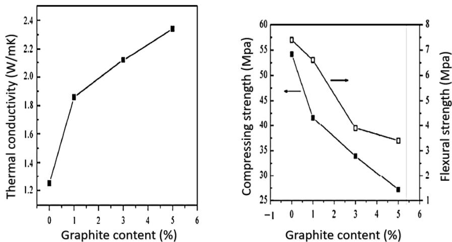
*Figure 10. the effect of graphite content on thermal conductivity, compressive and flexural strength of concrete [96]*
