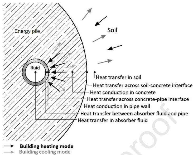
Figure 2. Heat transfer stages in an energy pile
