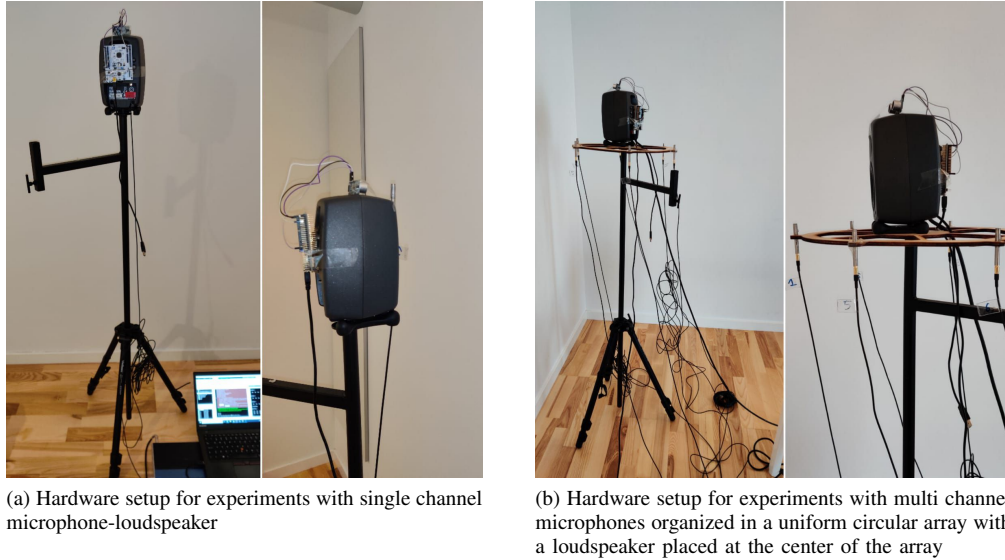
Fig. 1: Proof of concept used to obtain acoustic data
