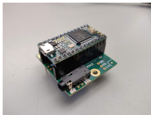
Figure 1. The Teensy 3.2 and its audio shield.
