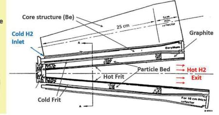
Power / Thrust: 260 MW / 48 kN
