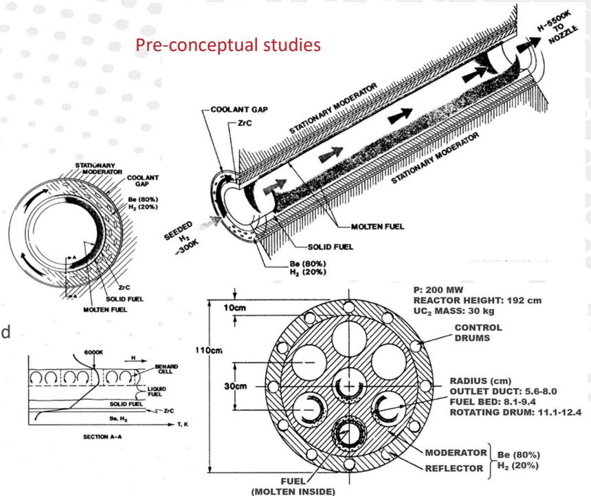
Fissioning fuel in plasma-like state at peak temperatures  $\sim 50\,000\text{ K}$
