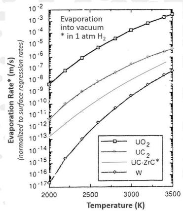
**W: the only known fully stable material in flowing  $H_2$  at  $T > 2500K \Rightarrow$  W-based Cermet fuel**
