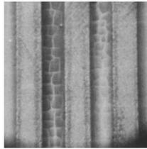
Cracks on the ZrC coating of coolant-channels (composite FE, NF-1 test)
