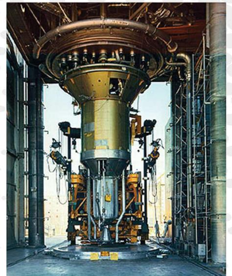
1140 MW nuclear reactor integrated in a complete mock-up of a nuclear rocket flight engine, tested in a simulated space vacuum
