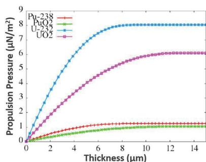
Propulsion pressure performance with  ${}^{232}\text{U}$  comparable to the one of solar sails near the earth (~9  $\mu\text{N}/\text{m}^2$ )
