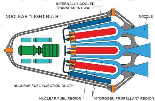
Ball of Uranium plasma (peak/edge temperature  $\sim 55\,000/26\,000\text{ K}$ ) hydrodynamically confined (vortex stabilized) by the flowing hydrogen propellant (which enters the cavity by flowing through its porous graphite wall)
