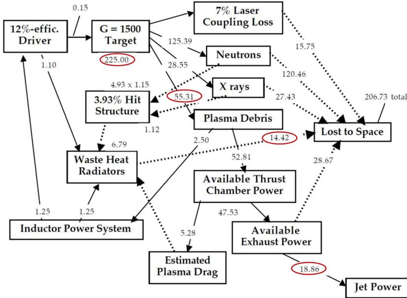
The jet power is ~8% of the power released by D-T fusion, and 15 times the laser driver power
