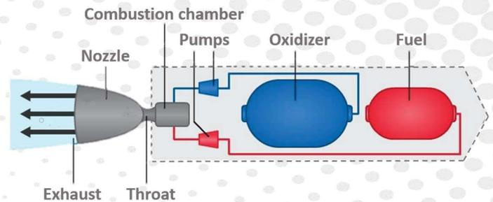
$$\text{Thrust} = \dot{m} v_{eject} + p_e A_e$$
