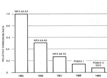
Improvements in relative corrosion rate of NERVA/Rover fuel elements
