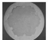
**BATH:** developed for the internal Shield of NERVA-derived engines (Al 70w%, TiH<sub>1.8</sub> 30w%, B<sub>4</sub>C 5w%)
