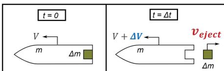
$$F_{thrust} = m \frac{dV}{dt} = v_{eject} \frac{dm}{dt}$$
