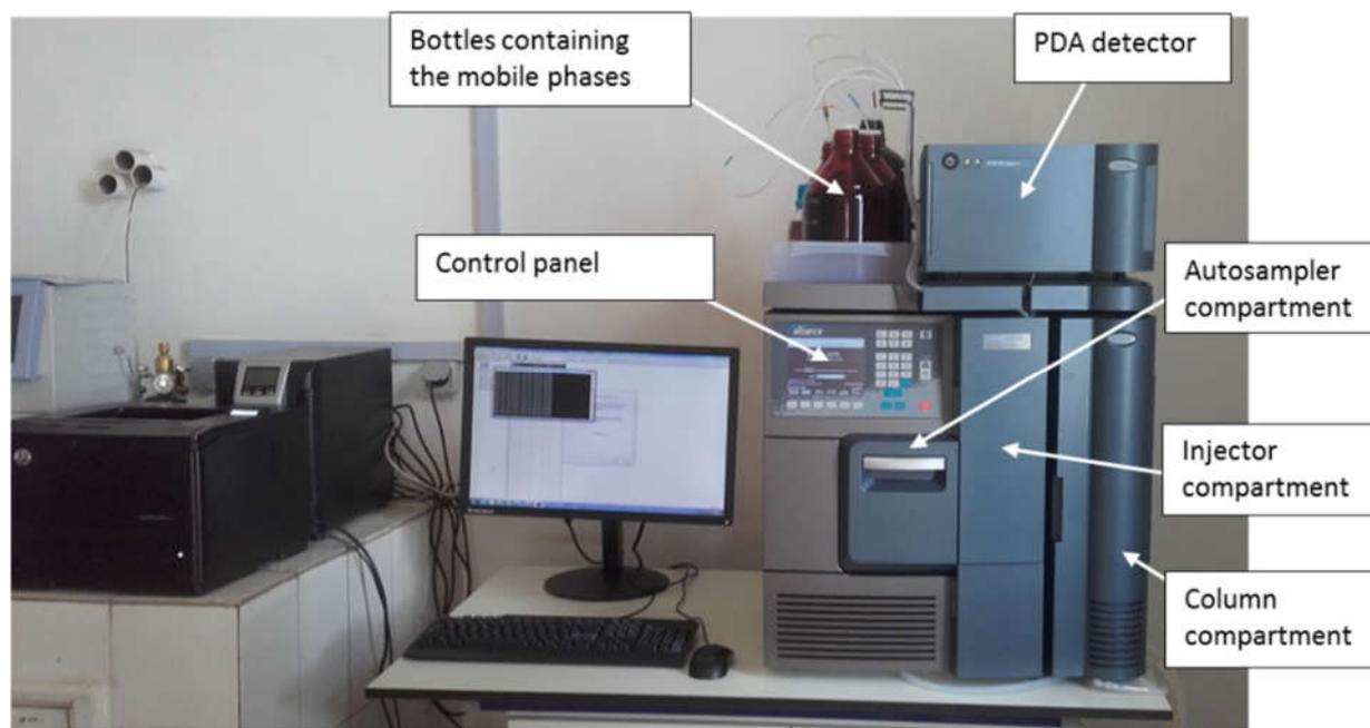
Figure 1: Picture of the Waters Alliance HPLC system installed in the LKMP lab at Cape Rubona.
